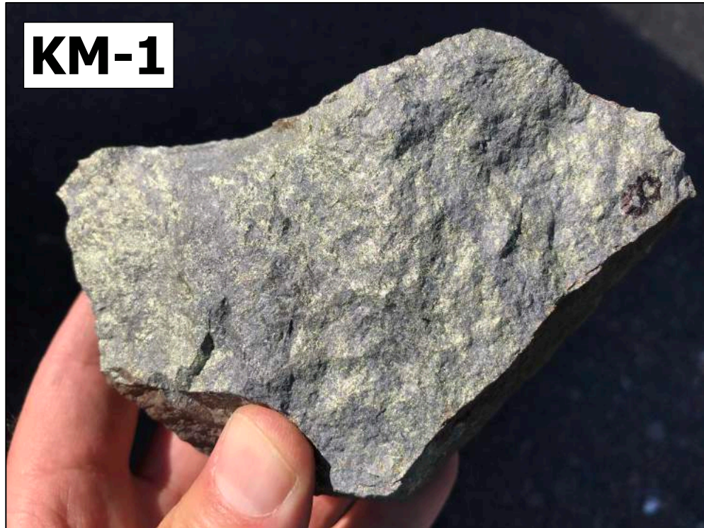
Figure 13. Massive sulfide mineralization collected by the author on mine dump at the No. 1 Shaft.
